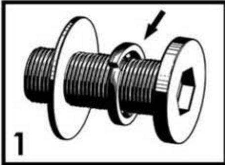
Before attaching each of the screws, make sure that the **smaller lock washer is between** the larger washer and the head of the screw.
